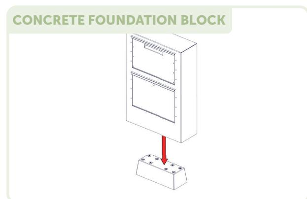
8. Secure the parcel letterbox to the paving or paving stone using plugs or chemical anchors. This is not necessary when securing to a concrete base.
